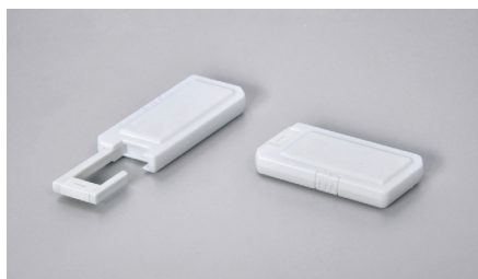
Snow White T183 Frequency : 8.2MHz/58KHz Dimension: 21mmx55mmx9mm Color: White or customized Packing: 40cmx38.5cmx33.5cm, 1800pcs/ctn, 19kgs/ctn
