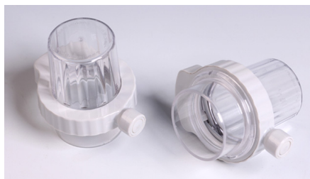
Easicap Big Straight NO.B009/B Frequency: 58 KHz/8.2 MHz/66KHz Dimension: Ø40.5mmx75mm Rang of protection: Ø31mm~36mm Color: Grey, Beige, Black or customized Lock: Standard/Super Packing: 58.5x39x34cm; 200pcs/ctn, 11.85kgs/ctn
