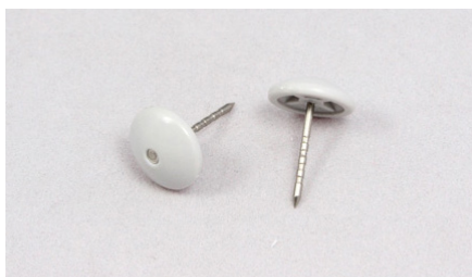
Mini No.P15 Length: 16mm/17mm/19mm Remark: Groove/Smooth Color: White/Black/Beige/Gray Head diameter: Ø13mm Packing: 34x25x17cm, 10000pcs/ctn, 5.7kgs/ctn
